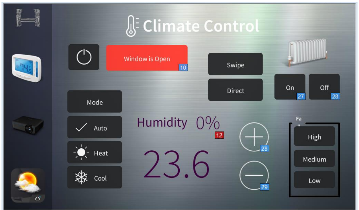
Figure 3.6. HVAC control system user interface
