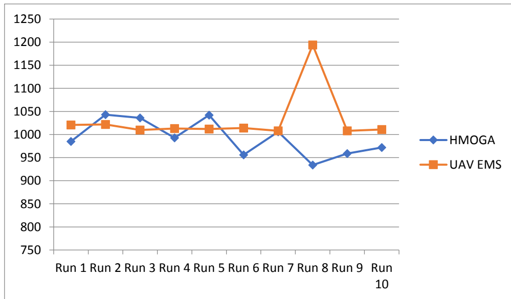
Figure 20. Comparison of average generation with the best fitness function in Scenario 6 of HMOGA and UAV EMS approach
