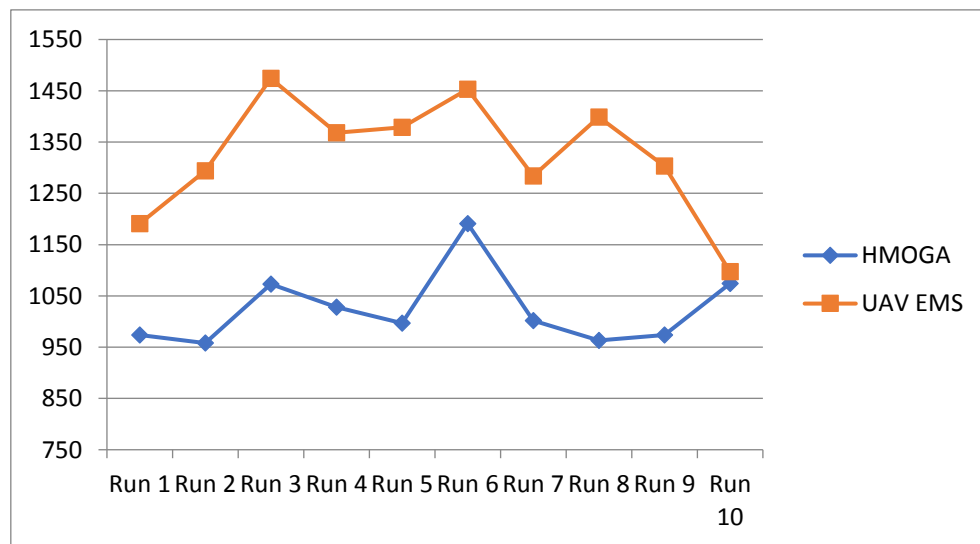
Figure 22. Comparison of average generation with the best fitness function in Scenario 8 of HMOGA and UAV EMS approach
