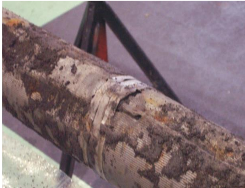
Figure 18. Screen failure-caused by high drawdown and plugging[10]
