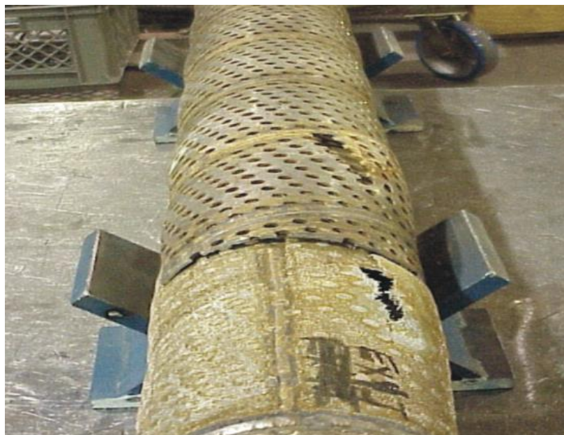
Figure 19. Screen failure-caused by non-sealing mechanical fluid loss device or poor injection well filtrations[10]
