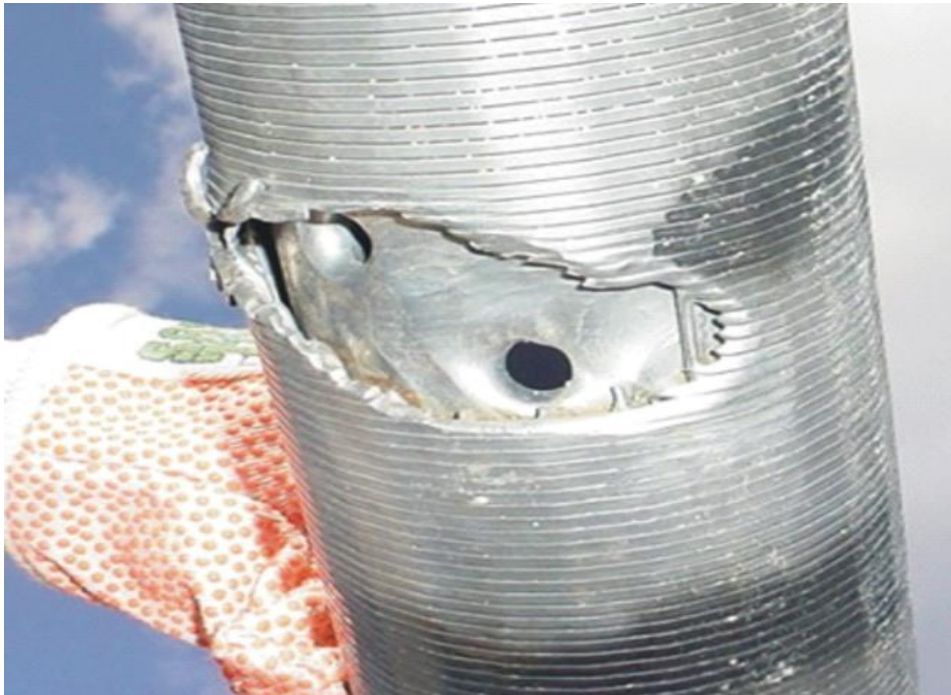
Figure 16. Screen failure-caused by erosion during pumping[10]
