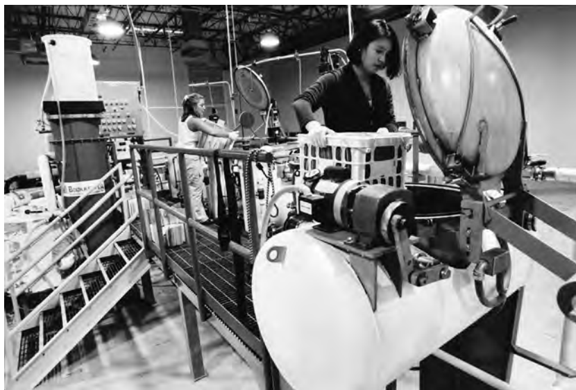
Fig. 2 Bookkeeper deacidification cylinder for archival materials. (Courtesy of Preservation Technologies, 2002.) Foreground shows loading archival materials in the horizontal cylinder while books are being prepared for the vertical book cylinder.
