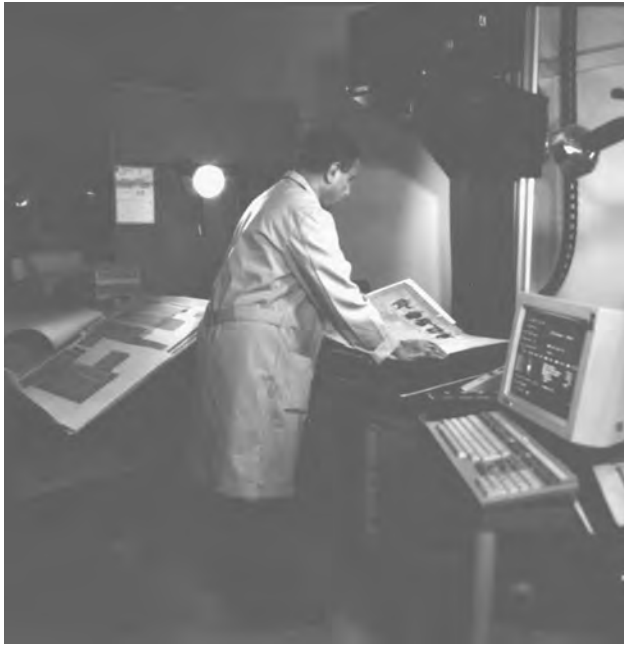
Fig. 5 Herrmann and Kraemer 35-mm camera and book cradle. (Courtesy of Preservation Resources, 2001.)
