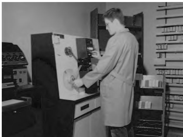
Fig. 10 Direct duplication of microfilm. (Courtesy of Preservation Resources, 2001.)
