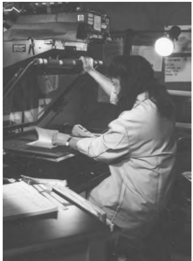
Fig. 4 Herrmann and Kraemer 35-mm camera filming of flat scrapbook collection. (Courtesy of Preservation Resources, 2001.)
