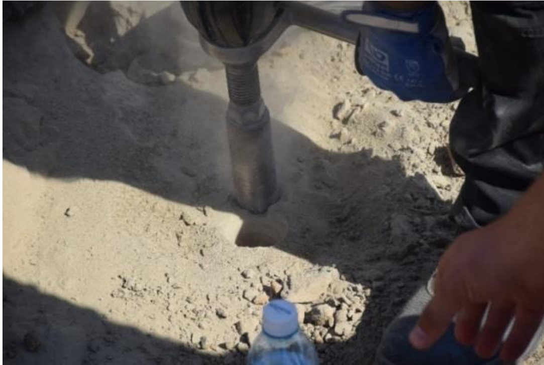
Figure 8. Procedure of sampling sister-plugs in proximity.
