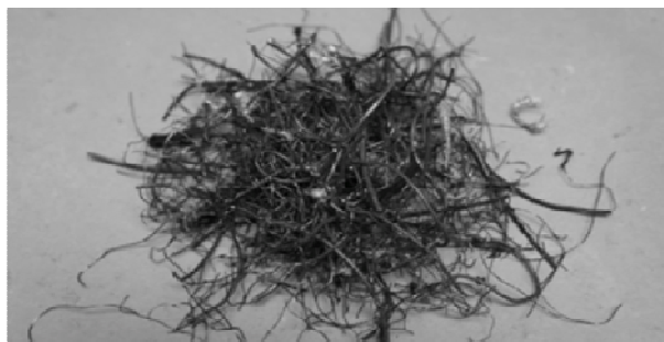
Figure 2. Recycled steel fibers extracted from rubber tires
