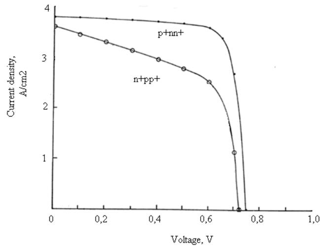
Fig. 2. A comparison of  $\text{p}^+\text{nn}^+$  cells and  $\text{n}^+\text{pp}^+$  cell performance; points – experiment.
