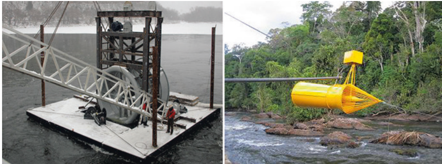
Fig. 12 Hydrokinetic turbines (Site: http://www.cerpch.unifei.edu.br/hidrocinetica.php ). a Hydrokinetic helical-type turbine (Darreus turbine). b Hydrokinetic helical-type turbine (Gorlov turbine)
