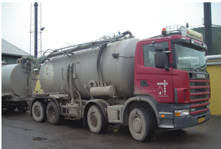
Fig. 5 Truck leaving the receiving unit at Hashøj biogas plant after delivering manure. It will return to the farms with digested manure (Photo by author, 2009)
