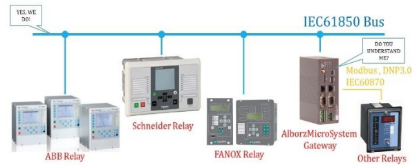
Figure 2 IEC61850 communication Standard and different IEDs communicating in a gateway
