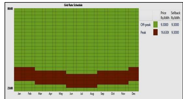
Fig 3. Grid rate schedule specified in HOMER Pro.
