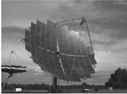
Figure 5.9 Solar System's Concentrator receiver designed for applications at 400\times – 500\times (Source: Solar Systems, reproduced with the permission of Sam Carter, Solar Systems)
