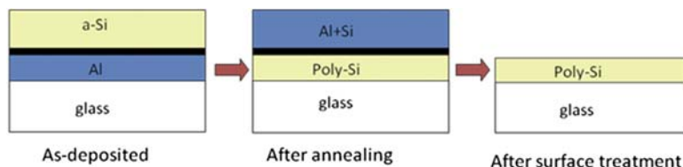
Figure 3.4 AIC process schematic where the thick black line represents the permeable interface between the Al and Si layers. Adapted from Fuhs et al. 27
