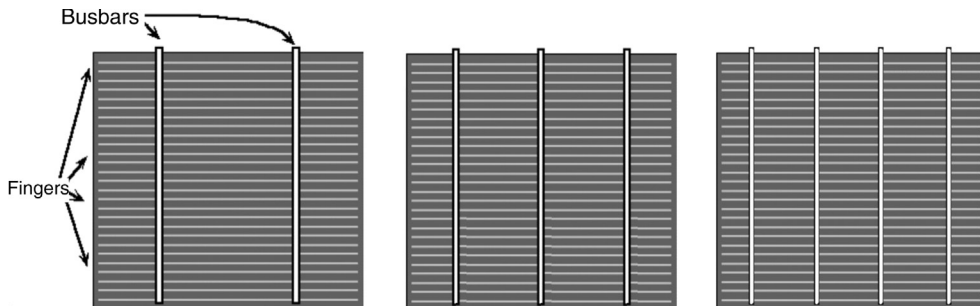
FIGURE 9.10 A comparison of front contact grid pattern for two, three, and four busbars.
