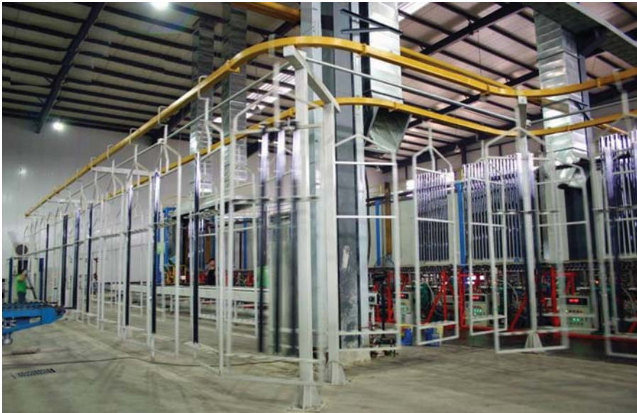
Plate 13. Fully automatic facility for manufacturing of evacuated tubes. Top: Automatic evacuating machine. Bottom: Automatic conveying line. This facility produces 20 million evacuated tubes each year. Courtesy of Himin Solar Energy Group, Dezhou, China.
