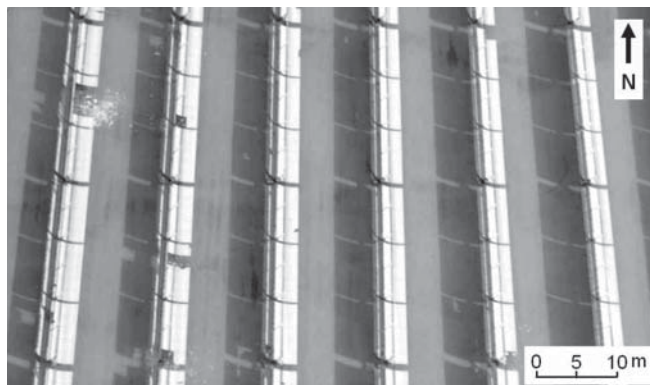
Figure 11.19 Aerial photo of SEGS system. The axes of the parabolic mirrors are north–south, which turn from east to west every day. About 3000 mirrors are replaced each year because of wind damage. Several damaged mirrors are shown in this photo. To avoid shadows from neighboring mirrors, the distance between adjacent mirrors is about twice the width of the mirrors.
