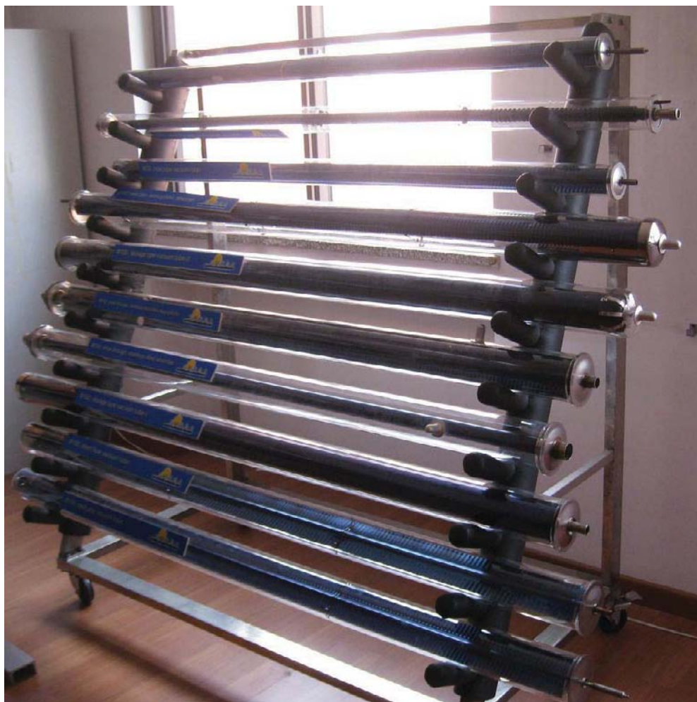
Plate 12. Various types of vacuum tube solar heat collectors. Currently, vacuum tube solar heat collectors are the most used solar heat collectors. They use selective coating to achieve maximum absorption of solar radiation, with minimum loss of heat by radiation. The vacuum between the outer tube and the heated element provides almost perfect thermal insulation. Depending on the ways of transferring heat, there are several types: The direct-flow vacuum tube heat collector allows water to flow by convection into the tubes. The heat siphon collector uses an ingenious phase-change mechanism to transfer heat with very high efficiency and prevents heat from flowing back to the tube (the thermal diode effect). See Section 11.2. Photo taken by the author. Courtesy of Beijing Solar Energy Research Institute.
