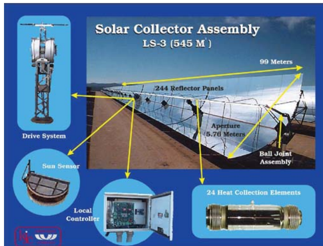
Plate 10. Solar collector assembly of a trough system. The axis of the parabolic troughs are aligned South-North. A tracking mechanism turns the troughs every day from East to West. The solar radiation is focused on the vacuum-tube heat collectors. The collectors heat synthetic oil to 400°C, then generates superheated steam to drive steam turbines. The highest efficiency on record was 20%. See Section 11.4.
