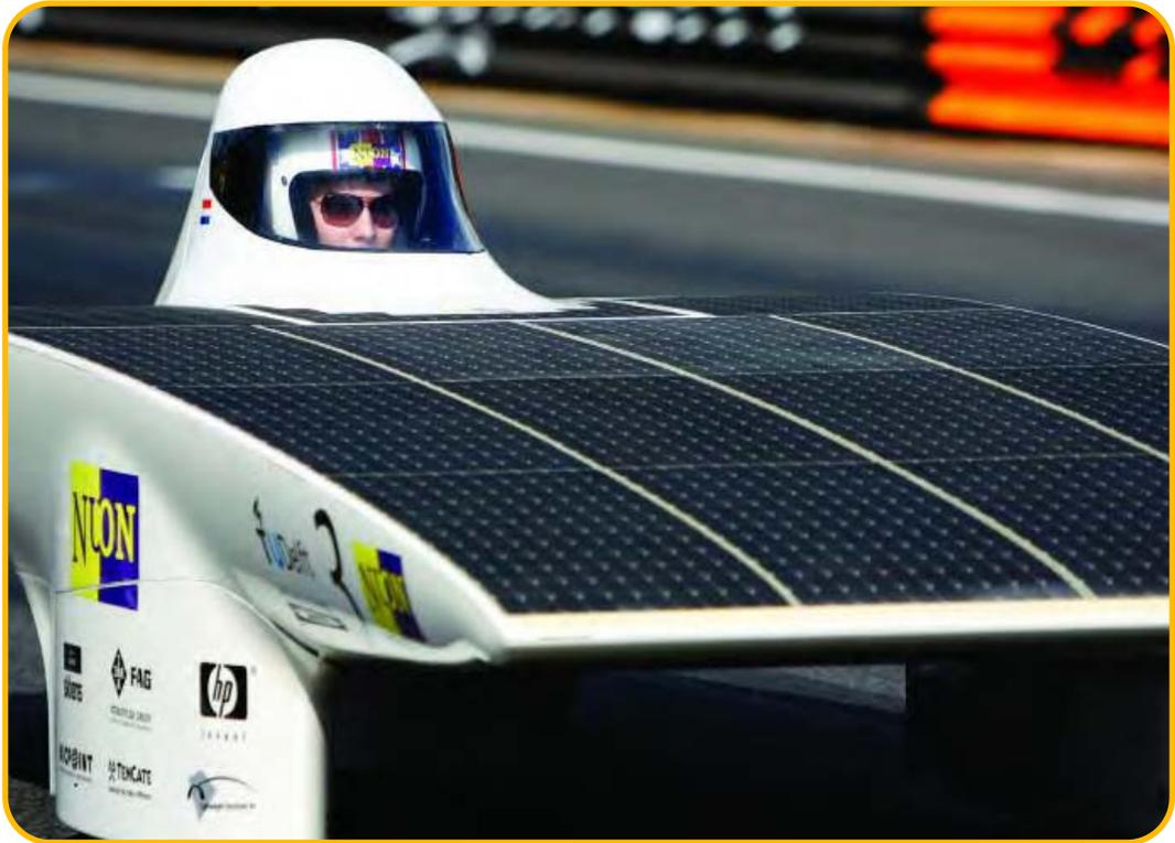
Unfortunately, solar cars are not ready to replace gas-powered vehicles. Solar cell efficiency limits their usefulness as transportation vehicles. Engineers and hobbyists build most solar cars to compete in speed and distance races around the world. To make cars as efficient as possible, they eliminate extra space and weight. The interiors usually have just enough room for a driver to squeeze in. The competitions promote solar technology and encourage builders to improve their machines.
