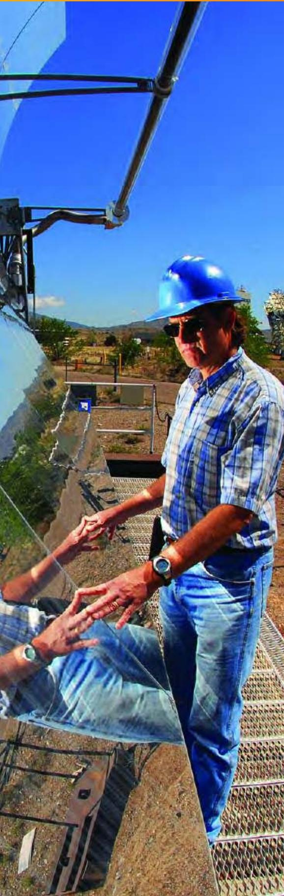
A **parabolic trough** is also a solar thermal collector. It is a long, curved shiny panel, or mirror. Solar thermal power plants use rows and rows of them. Trough collectors direct sunlight to tubes that run down the center of the troughs. A liquid, such as oil, flows through the tubes and transfers heat to produce steam. Solar thermal power plants use steam to drive the blades of a **turbine**. The turbine transfers energy to a **generator**, which produces electricity.
