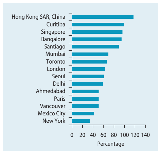
FIGURE 3.4 Ratio of public transit fares to operating costs in a sample of large cities
